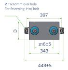
Connector for 1 or 2 wires 6 sqmm to 50 sqmm Maximum torque: 2.77kgf.m
